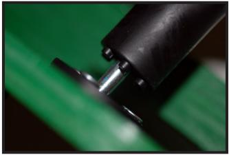
**Step 3**Attach the cylindrical pivot post piece to the circular pivot post adapter. The protrusions from the cylinder should fit in the holes on the circular piece.
