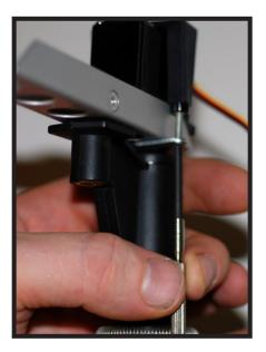
**Step 8**Wrap the plastic cradle around the servo, and feed the attached metal bracket underneath the metal link. Tighten the screws.
