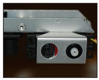
**Step 10**Place the 2-hole metal link over the servo you just attached. Note: This image depicts a HS-422 servo, but you should have a HS-645MG servo installed here.
