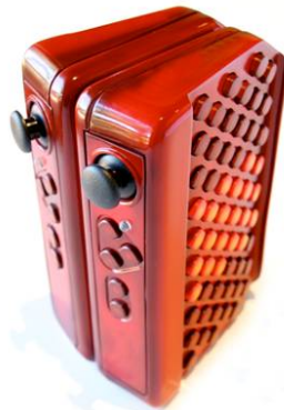
Figure 1: Thumtronics forthcoming USB-MIDI controller, the Thummer, contains two keyboards, each with 57 pressure-sensitive buttons. A variety of controllers include two thumb-operated joysticks and optional internal motion sensors. One side of the Thummer layout is used to concretely demonstrate the possibility of tuning and transpositional invariance.
