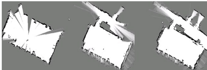
Figure 2.5.2.2 The mapping process, all information fused into a 2D global map
